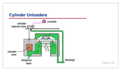
In response to an increasing load, the controller sends a signal to close the solenoid valve. This closes the port that allows the pressurized refrigerant vapor to travel to the top of the unloader valve. A controlled leakage rate around the unloader valve relieves the pressure, allowing the valve to open and refrigerant vapor to once again flow to the cylinder to be compressed.
